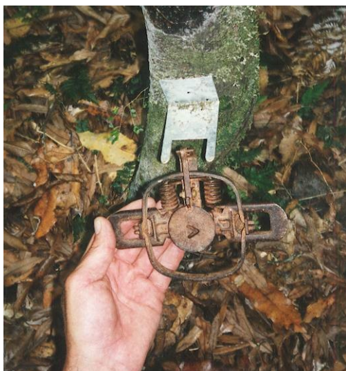
No. 1 leg-hold trap shown with bracket for raising the trap above the ground. Photo courtesy Pest Control Research Ltd
